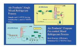
For 2 MTPA plants, a Propane Pre-cooled Mixed Refrigerant (C3-MR) process is applied because of its improved energy efficiency.
